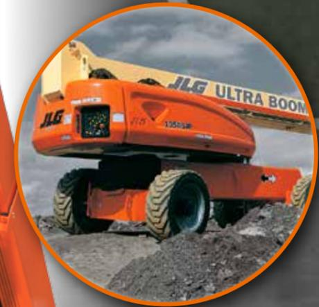
Conquer Rough Terrain with the tightest turning radius, best crab steer ratio and only oscillating axle in its class, you can go where other boom lifts simply can't.
