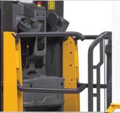
**3 DRIVER SAFETY SYSTEM** Automatic stop if side gates are not lowered when driver platform above 1200.
