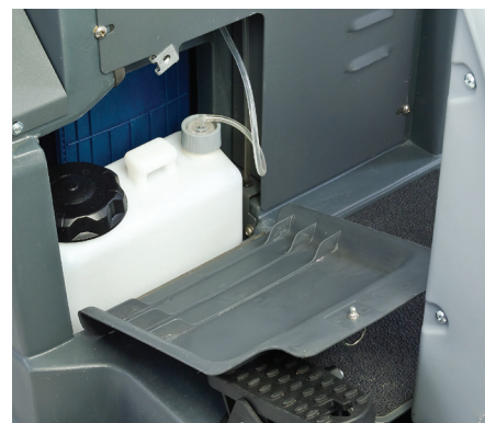
Easy change of cartridge, now located underneath the seat
