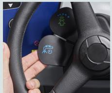
Intermittent SmartFlow™ lever integrated into steering wheel: Reduces water flow on the deck, preventing splashes during turns, lowering consumption and ensuring perfect drying performance
