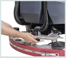
The squeegee is designed to be easily removed from its support using ergonomic handles and there is no hose connection/disconnection needed
